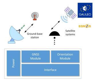
Fig. 4 Positioning receiver block diagram
