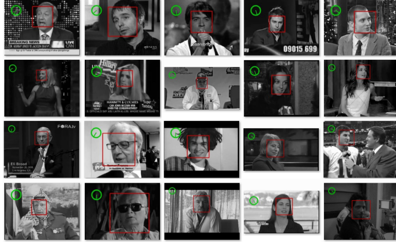
Fig. 1. Sample detections from the YouTube faces dataset. The red rectangle depicts the detected face, and the estimated yaw angle is indicated inside the green circle at the top-left corner. The circle represents a top view of the face, and the green line inside it shows the detected yaw angle. A detected angle of 0^\circ is indicated by a line pointing downward. Despite the images having different backgrounds, presence of eye glasses or not, or some occlusion on the face, our method can predict the head pose correctly
