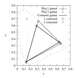
Figure 9. Common gamut and verification for two test projectors
