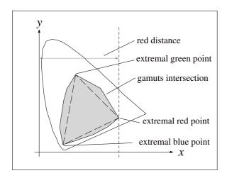
Figure 5. Extreme chromaticity points in the gamut intersection. The red distance to maximize is given as an example.
