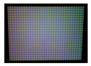
Figure 2. Location of the 825 shading points over the projected surface (one beamer)
