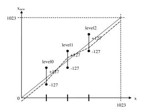
Figure 3. Shading correction for a single shading point
