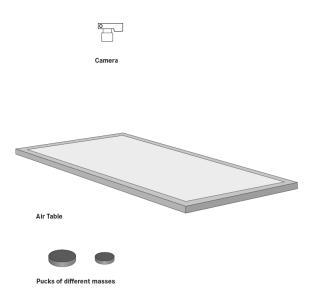
Fig. 1. The initial setup of the airtable experiment in the physics lab with a camera on top of the table recording the movement of the pucks.
