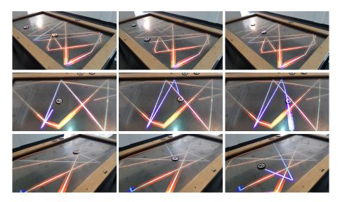
Fig. 5. Visualization of the markers movement on the air table. High velocity(angular velocity) is mapped to red(yellow) and low velocity(angular velocity) to blue(light blue)
