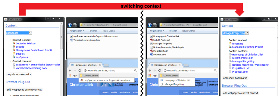
Fig. 2. Screenshot showing sidebar, file explorer and browser before (left half) and after a context switch (right half), illustrating the effects of a dynamic reorganization of the system. (Note: windows were rearranged for easier comparison.)
